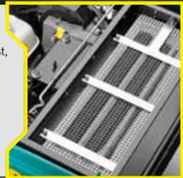
The battery operated version boasts a superior running time, for extra productivity. Maintenance access is convenient as well. The top lifts up to expose the engine or the battery compartment as well as motors and other service areas.
